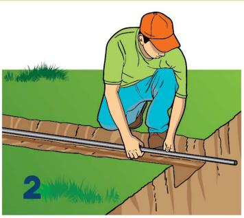
Bury the one-inch PVC pipe that runs from the laundry, bathroom or kitchen to the hole.
