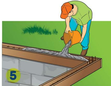
On top of the last row of blocks, place the mould for the capping beam and fill with concrete.
